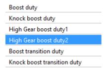
Nissan sense gear position by comparing RPM to vehicle speed (there is no switch on the gearbox to indicate gear position to the ECU). Use the boost coefficient parameters to adjust the speed/RPM ratio where necessary. There are differences in calculations of low/high gear between auto and manual vehicles.
